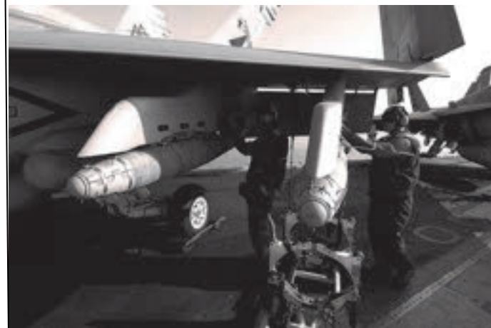
Arabian Gulf (Nov. 9, 2004) — Aviation Ordnancemen, assigned to the "Rampagers" of Strike Fighter Squadron Eight Three (VFA-83), finish loading two of the Navy's latest Satellite Guided Bombs, the GBU-38, aboard the aircraft carrier USS John F. Kennedy . The GBU-38 is a 500-pound Joint Direct Attack Munition (JDAM is a guidance kit that converts existing unguided bombs into precision-guided "smart" munitions; the tail section contains an inertial navigational system and a global positioning system) that uses a standard Mk-82 bomb, and was developed for precision bombing in urban warfare. Carrier Air Wing Seventeen (CVW-17) aircraft aboard Kennedy are supporting ground troops in Fallujah, Iraq, under Operation Al Fajr (New Dawn). (U.S. Navy photo)
