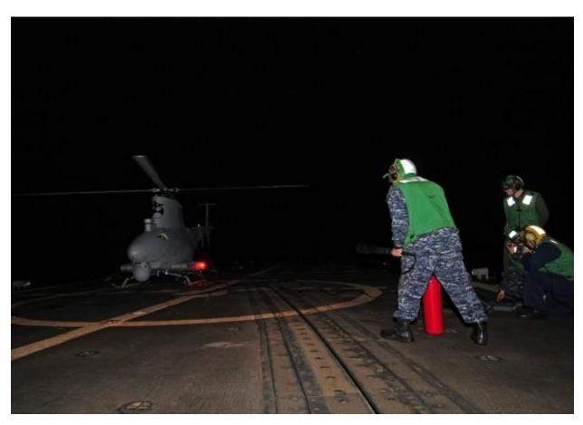
An MQ-8 Fire Scout robot helicopter lands aboard the Navy frigate USS Simpson off the African coast this year. Photo: Navy
